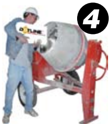
4 With mixer still turning, add pre-determined units of DOTline™. Mix for 1 minute Add in remaining 1 quart of water per each unit of DOTline™ used.
